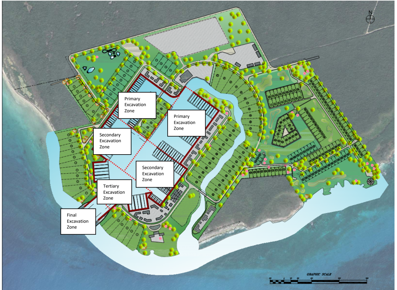
Figure 186. Conceptual Basin Excavation Phasing (Red – Impermeable Bulkhead; Dashed Line – Temporary Cut-off Wall).
