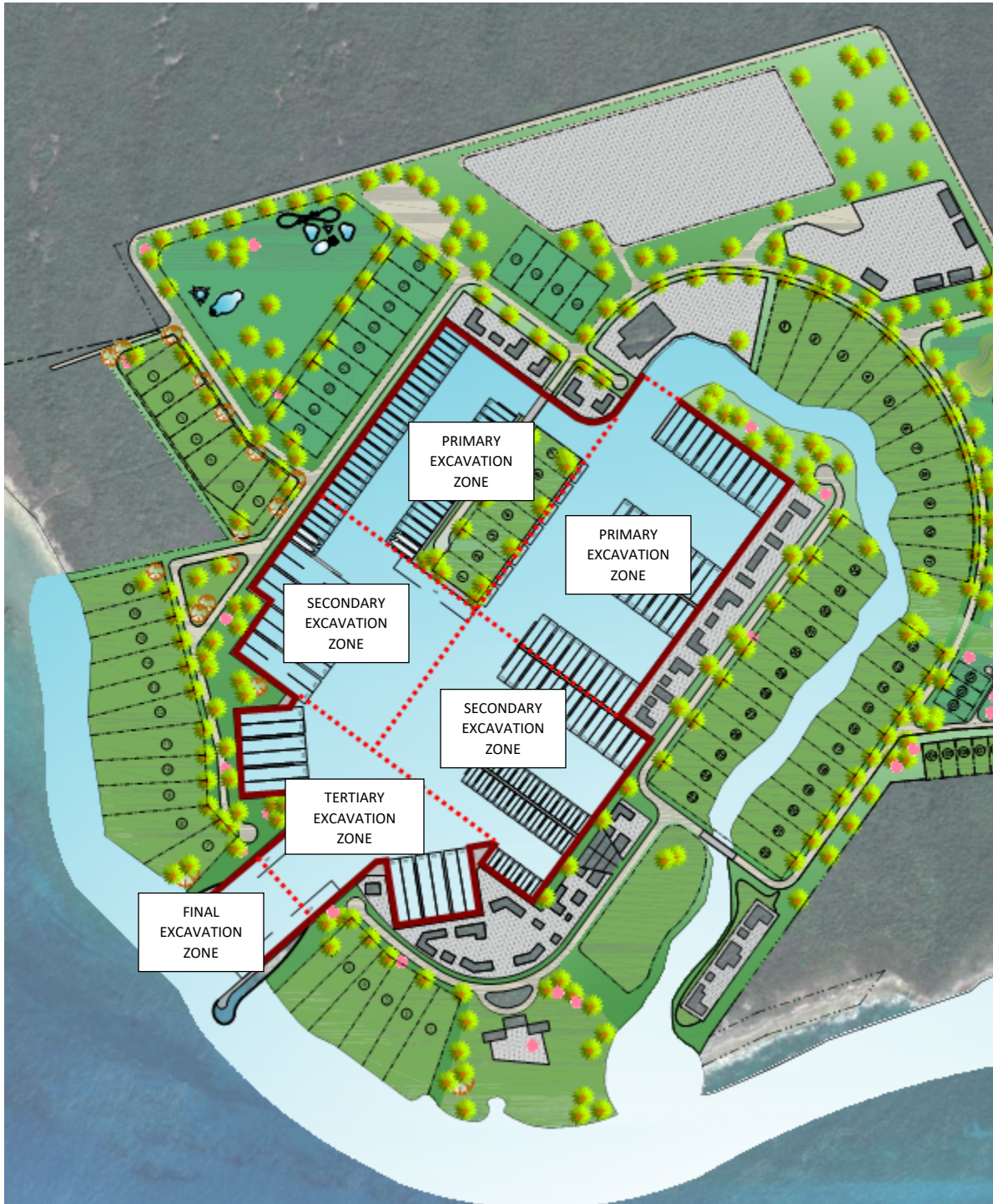
Figure 5. Conceptual Basin Excavation Phasing (Red – Impermeable Bulkhead; Dashed Line – Temporary Cut-off Wall)
