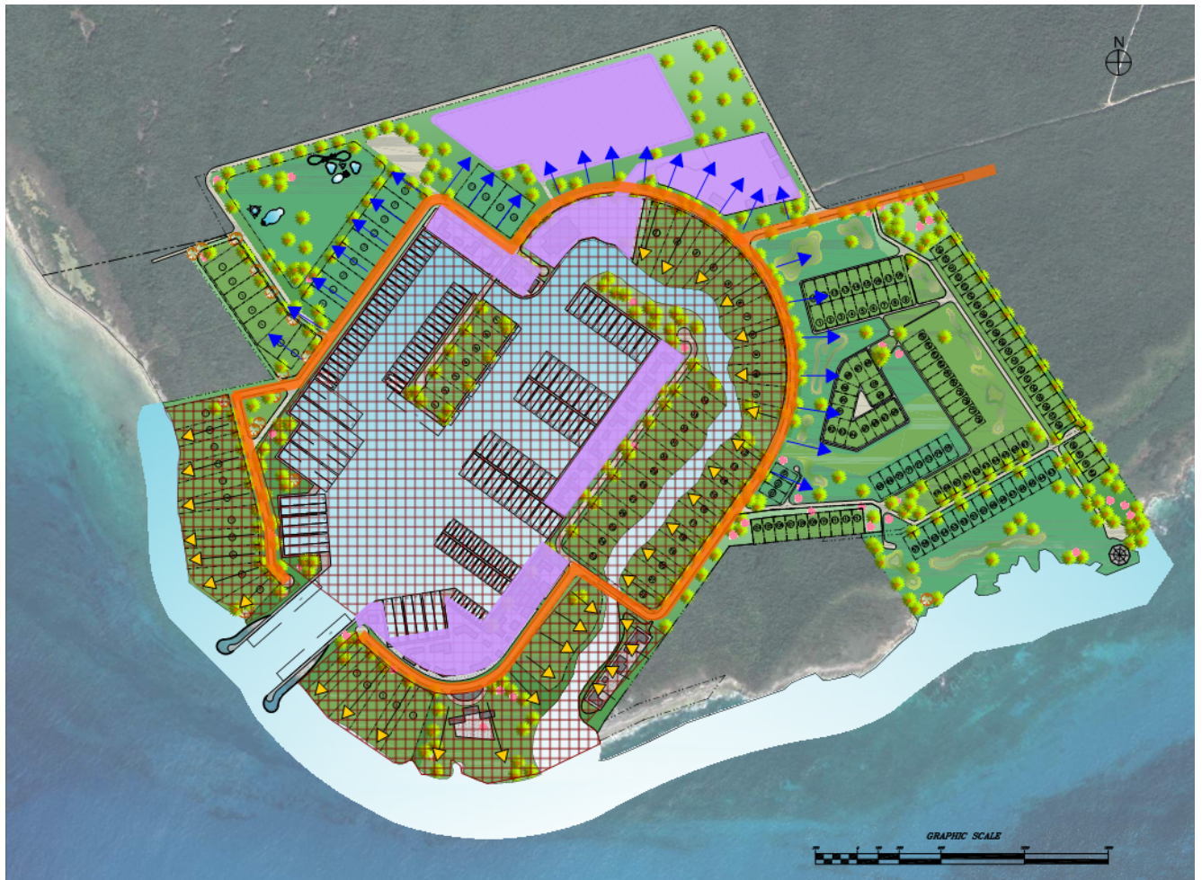
Figure 187. Storm Surge Management Plan (Blue Arrows – Net Rainwater drainage direction; Yellow Arrows – Net Seawater and Rainwater drainage direction; Orange – Perimeter Road; Purple – Special Drainage Design Areas, Hatched Area – Localized Storm Surge Management Zone).
