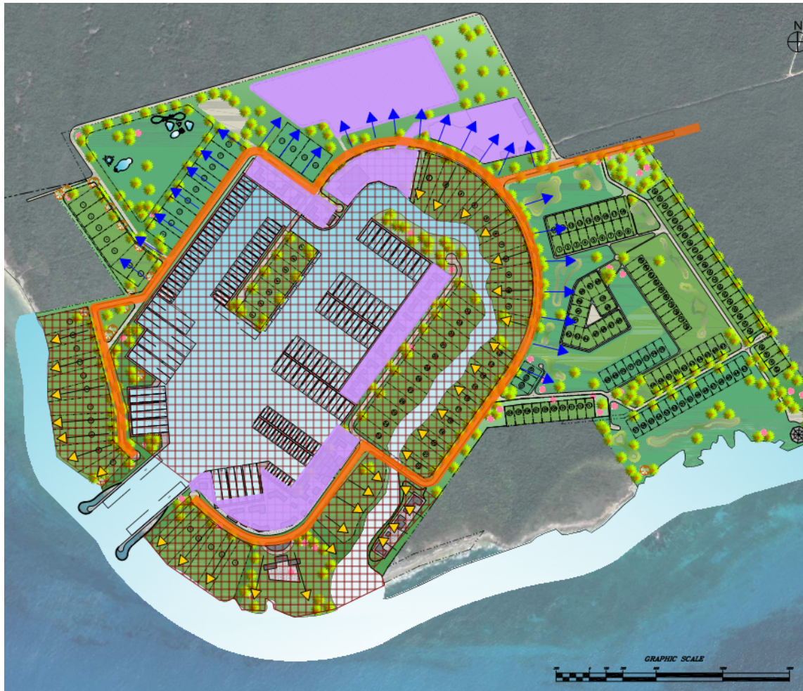
Figure 6. Storm Surge Management Plan (Blue Arrows – Net Rainwater drainage direction; Yellow Arrows – Net Seawater and Rainwater drainage direction; Orange – Perimeter Road; Purple – Special Drainage Design Areas, Hatched Area – Localized Storm Surge Management Zone)
